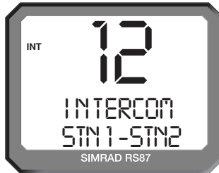
Fig 6.7 - Interkom-Ruf von Station 1 an Station 2
